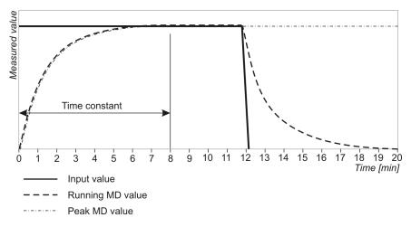
Figure 9: Operation of thermal MD function
