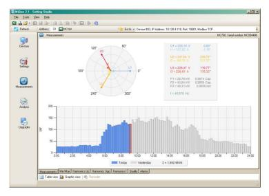
**Figure 26:** Online measurements in graphical form – phaser diagram and daily total active power consumption histogram
