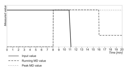
Figure 10: Operation of Fixed window MD function
