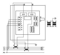
Connection 3u (2W3) Three-phase – threewire connection with unbalanced load
