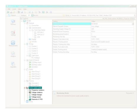
**Figure 24:** Settings for power quality parameters are set with setting and monitoring software MiQen
