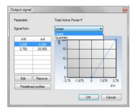
Figure 14: MiQen window for output signal definition
