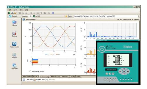
**Figure 28:** Online harmonic measurements in graphical form and interactive instrument
