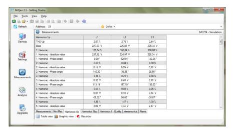
Figure 34: Tabelaric presentation of phase voltage harmonic components
