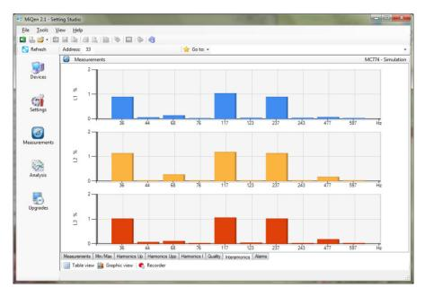
Figure 37: Graphical presentation of phase voltage interharmonic component
