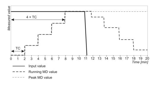
Figure 11: Operation of Sliding window MD function
