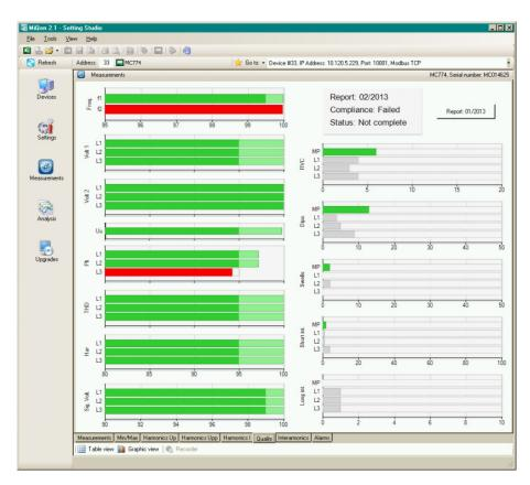
**Figure 39:** Graphical presentation of PQ parameters and overall compliance are available only for actual monitoring period
