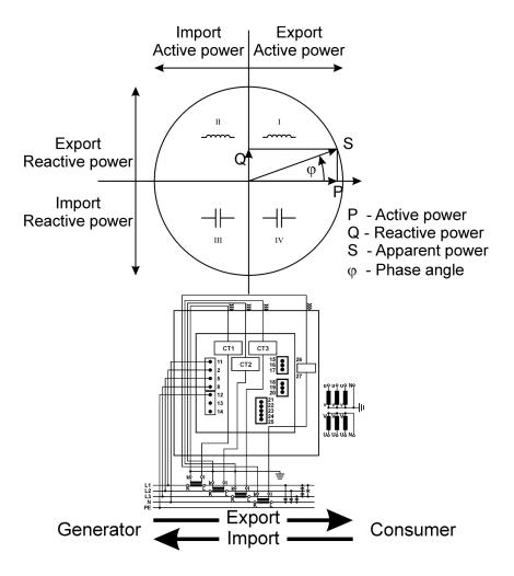
Figure 29: Explanation of energy flow direction
