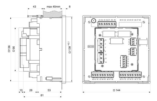
Figure 1: Dimensional drawing and rear connection terminals position
