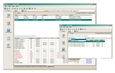
**Figure 42:** By clicking on "Show details" for each PQ parameter MiQen displays time-stamped measurements (events), which were outside limit lines
