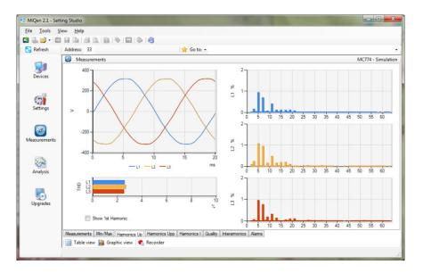
Figure 35: Graphical presentation of phase voltage harmonic components
