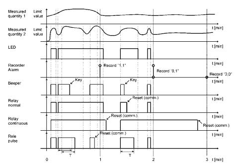
Figure 18: Graphical presentation of alarms operation
