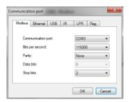
Choose correct communication interface (Modbus, Ethernet or USB) and set correct communication parameters.
