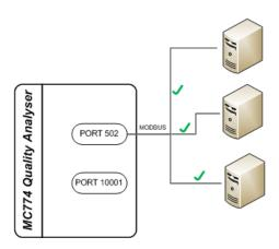
**Figure 12:** Multiple connections to a device are possible when port 502 (special MODBUS port) is used
