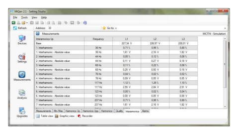
**Figure 36:** Tabelaric presentation of 10 phase voltage interharmonic components
