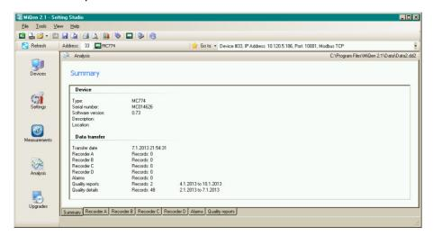
**Figure 40:** Information about downloaded data with tabs for different memory partitions
