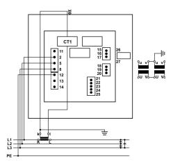
Connection 3b (1W3) Three-phase – threewire connection with balanced load
